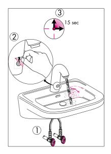
**Model 15180 only**: Pivot the temperature control lever forward to make the water cooler.
